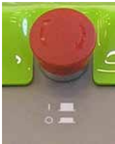
EMERGENCY PUSH BUTTON
