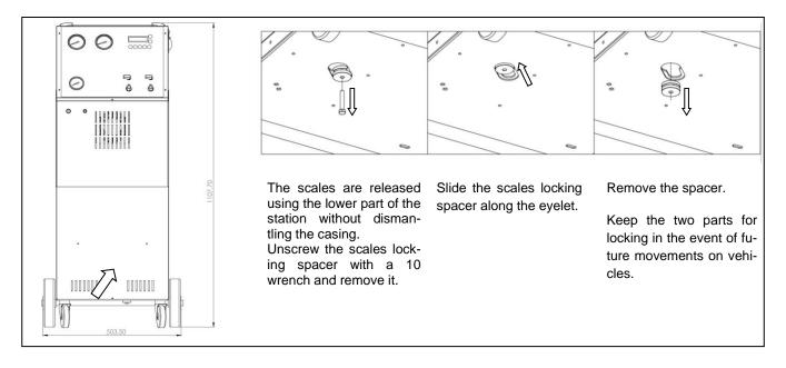
To avoid irreparable damage on the scales it is compulsory to block it again in the event the machine has to be transported on vehicles.
